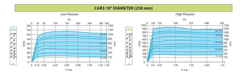
Airflow measurements taken at 68°F (20°C) at 1 atmosphere pressure.
