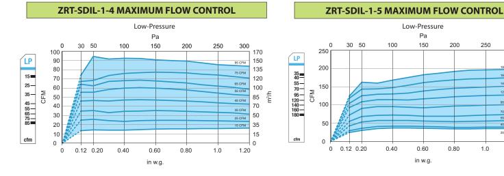
Airflow measurements taken at  $68^{\circ}F(20^{\circ}C)$  at 1 atmosphere pressure.
