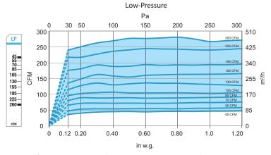
Airflow measurements taken at  $68^{\circ}F$  ( $20^{\circ}C$ ) at 1 atmosphere pressure.
