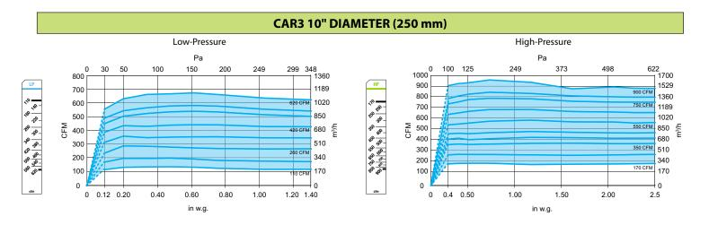
Airflow measurements taken at 68°F (20°C) at 1 atmosphere pressure.
