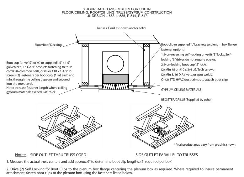
Note: When Non-Drive boot clips or supplied 1.5" x 1.5" galvenized, 16 gauge "L" brackets are used, fasten boot clips to the plenum box flange using a minimum of (2) #8 or #10 x 3/ 4 Lg sheet metal screws, (2) 3/16" diameter rivets, or (2) spot welds, for each boot clip.
