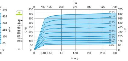
Airflow measurements taken at 68°F (20°C) at 1 atmosphere pressure.
