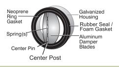
8" - 16" MODELS ROLLED METAL SLEEVE / CENTER POST DESIGN
