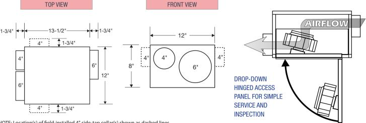
NOTE: Location(s) of field-installed 4" side-tap collar(s) shown as dashed lines.
