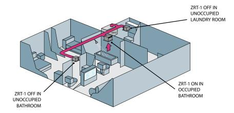
Eliminate the need for multiple noisy, inefficient spot fans by consolidating everything into a single effective system. The kit contains an energy-ZRT-1s for zone-controlled spot ventilation. Air is only drawn from bathrooms in use. The kit can be used for homes with 2-5 bathrooms, and expansion kits are available. \*Compatible with ZTC and MPVS150 Ventilator; sold seperately.
