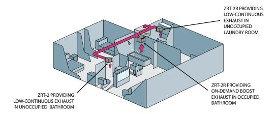
Using ZRT-2s to provide low-continuous IAQ ventilation and zone-based on-demand boost ventilation for homes with 2-4 bathrooms. This kit is designed to meet ASHRAE 62.2, ENERGY STAR with IAP, LEED for Homes, and California Title 24 standards. \*Compatible with MPVS150 Ventilator; sold seperately.
