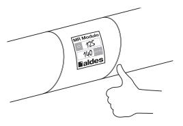
Write the diameter and airflow setting on the provided sticker and place it directly onto the duct to show where the MR Modulo has been installed.
