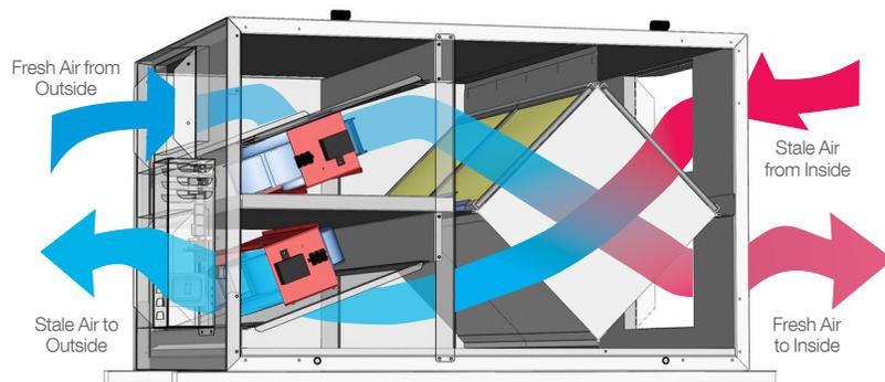
In the heating season, Heat Recovery Ventilators (HRV) and Energy Recovery Ventilators (ERV) draw in fresh air from outside while stale, humid air is exhausted. As the fresh and stale airstreams pass through the unit's core, the fresh air is tempered with heat recovered from the exhaust air. In the cooling season, fresh outdoor air is cooled by the air-conditioned exhaust air. An ERV will also transfer moisture to improve comfort in homes.
