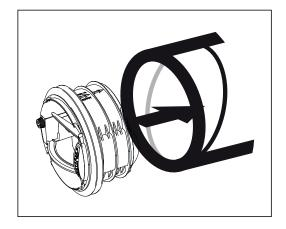
Orient the CAR3 according to the airflow direction indicated on the device. Horizontal or vertical mounting is acceptable.
