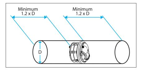
Regulator must be installed in a metallic air duct as pictured above. D represents the regulators maximum outer diameter.
