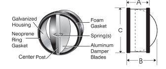
**NOTE:** Position of post in sleeve and number of springs varies according to model.
