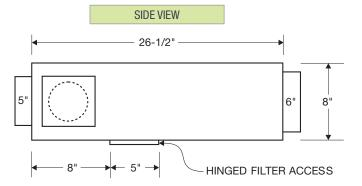
NOTE: Dashed lines indicate field installed side collar location
