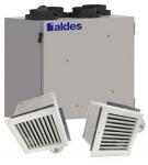
Energy Recovery Ventilator with Zone Register Terminals (ZRTs) for continuous IAQ exhaust and on-demand boost exhaust. Each ZRT is installed in one bathroom in the house. These kits transfer sensible and latent energy from stale exhaust air to fresh supply air. Kits are available for ventilating from 2-5 bathrooms.
