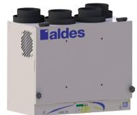
In the cooling season, the reverse occurs. The air exchanger cools incoming warm fresh air using the air-conditioned exhaust air from inside the home. Again, no mixing of the air steams take place. An ERV will also remove humidity from the warmer incoming air and transfer it to the drier outgoing exhaust air. This process reduces the humidity load on the air conditioning system, which would otherwise result in the continuous introduction of humid summer air to the home.
