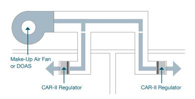
CAR-II's are used to control the amount of outside air brought into a building when installed in dedicated outdoor air systems (DOAS), make-up air fan systems, and AHU outside air plenums. This guarantees a delivered airflow rate and prevents over-ventilation in windy conditions.
