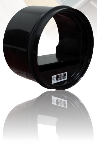
The CAR-II compensates for changes in duct pressure caused by thermal stack effect, building pressure, dust-clogged filters, etc. The CAR-II also provides a low-cost solution to balancing forcedair systems for heating, air conditioning and ventilation, eliminating the need for on-site balancing. The CAR-II will regulate airflow in supply, return, or exhaust duct systems.
