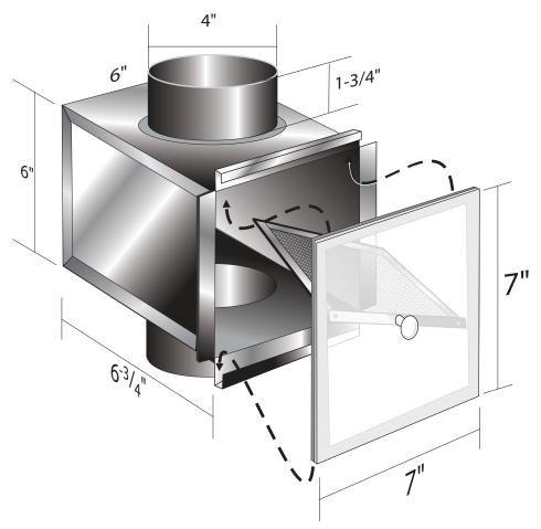
FOR DRYWALL INSTALLATION – CEILING OR WALL MOUNTED
