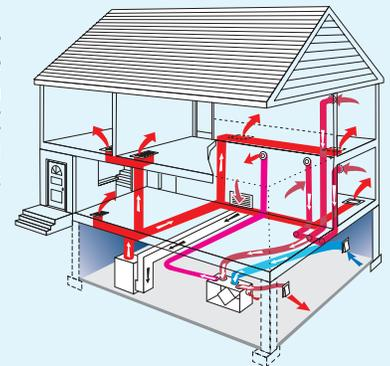
**Exhaust from H/AC Return and Distribution of Fresh Air through H/AC System**
